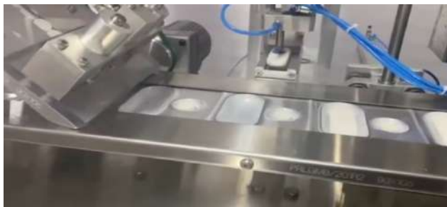
Fig. 2. Feeding device in blister machine
