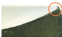
Figure 2. Example of the formation of J-shaped hooks on the edge of the punch
